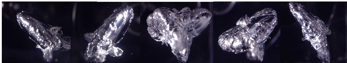
Figure 3.15 Final cavity morphology. Optical images of cavities in silicone (crosslinker mass fraction, f_x = 0.019 ) that illustrate more pronounced crack lobe formation with increasing oil content. Cavities are approximately 6 min after pulse initiation.
