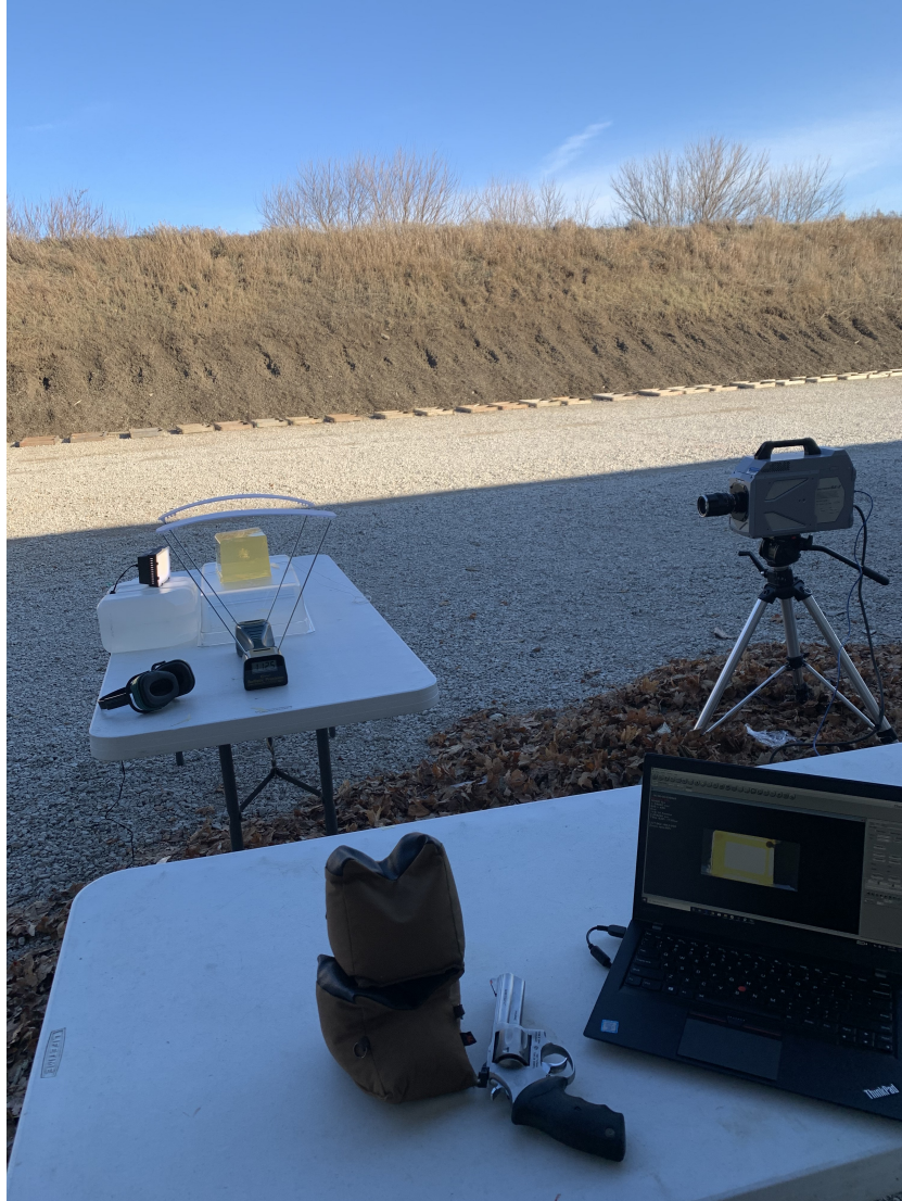
Figure 5.1 Firing range at Police Training Institute Tactical Training Center. The high speed camera captures images orthogonal to the projectile trajectory, with backlighting to enhance contrast. A chronograph (Caldwell) measures the projectile velocity just before impact with the gelatin
