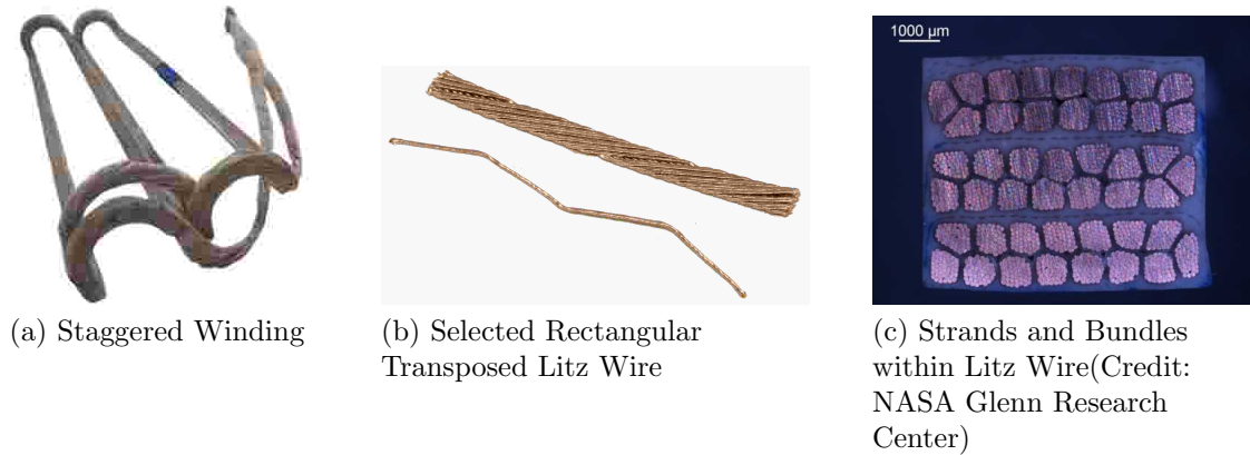
Figure 4.1: Form-Wound Winding and AWG 38 Litz Wire
