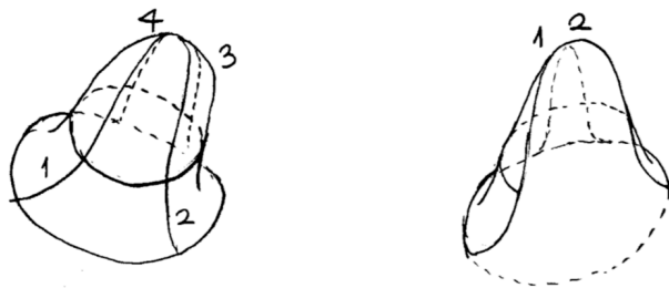
Figure 7b. Four nodal meridians and one nodal circle on the whole bell surface (left) and half meridians (right).
