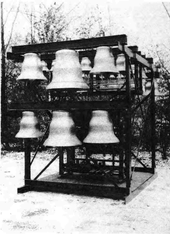
Figure 24a. First carillon with major-third bells made by using the FEM by Royal Bell-Foundry Eijsbouts 121
