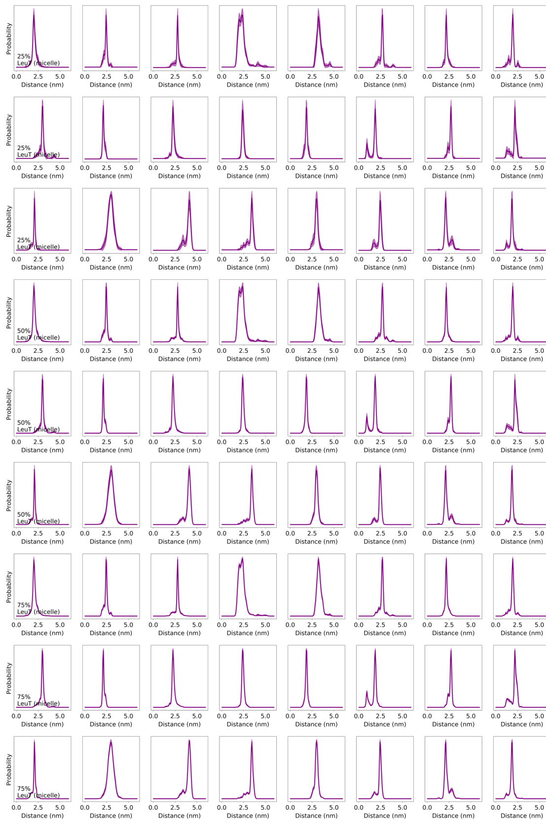
Supplementary Figure 5.6: Residue pair distance distributions for LeuT simulations in BDDM micelle averaged over 25%, 50%, and 75% of the collected trajectories. Filled regions show error bars in the distance distribution as obtained from 10 iterations where a subset of the trajectories are selected randomly.
