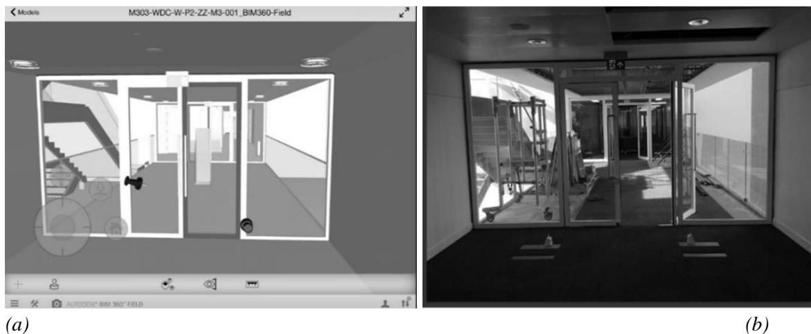
a) View of the Information Totem in yellow from the cloud based federated BIM model. b) Photograph of the same location on site as cross reference retrieved from the information totem.
