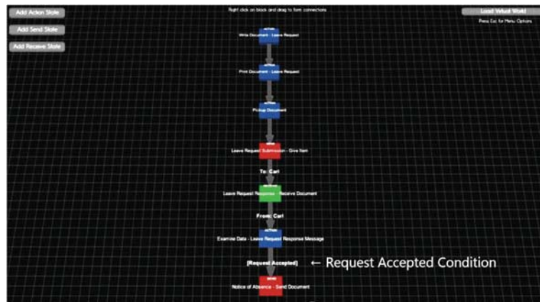
Fig. 7.7 Using the tool to specify choice in the world, showing the original S-BPM diagram, annotated to show choice insertion point
