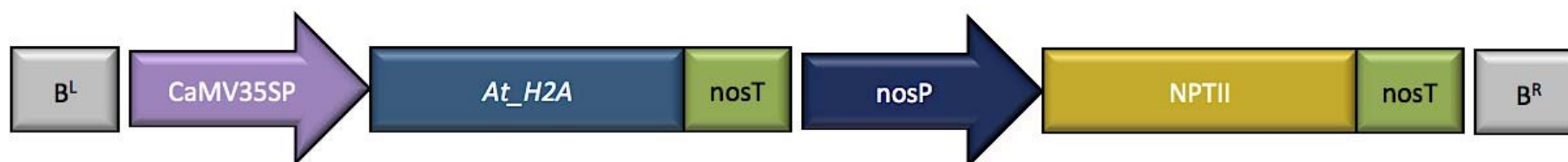
Figure 4.1 Schematic diagram of pBIN-35S-At_H2A vector T-DNA
