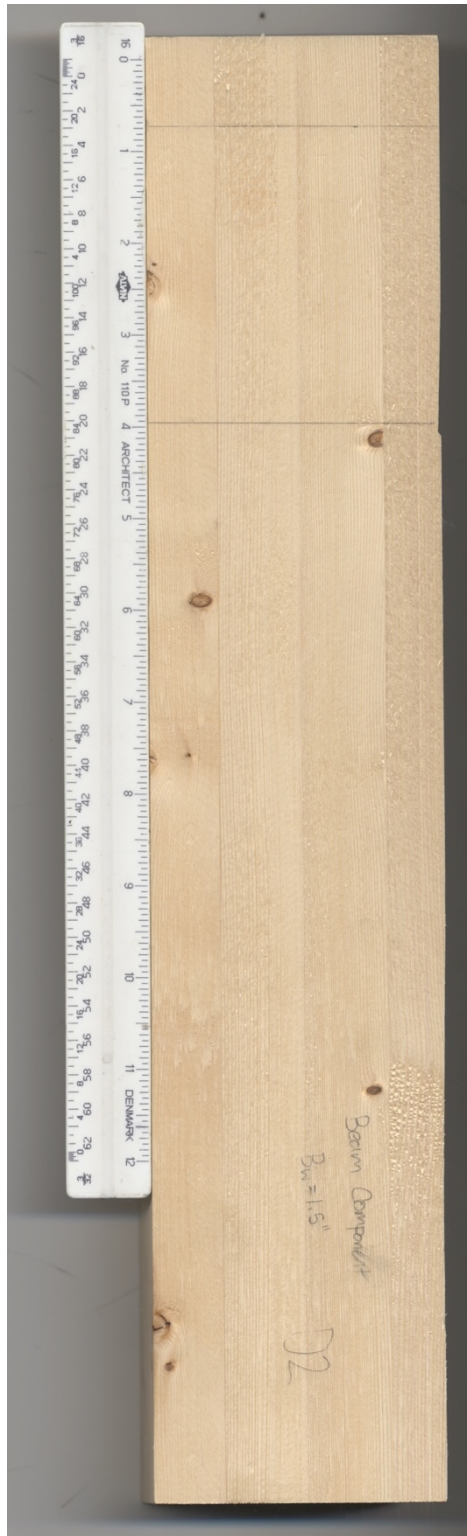
Figure 60. Specimen 2 of the glulam Nuki joint of B_w = 1.5'' , scanned after rotational stiffness testing.
