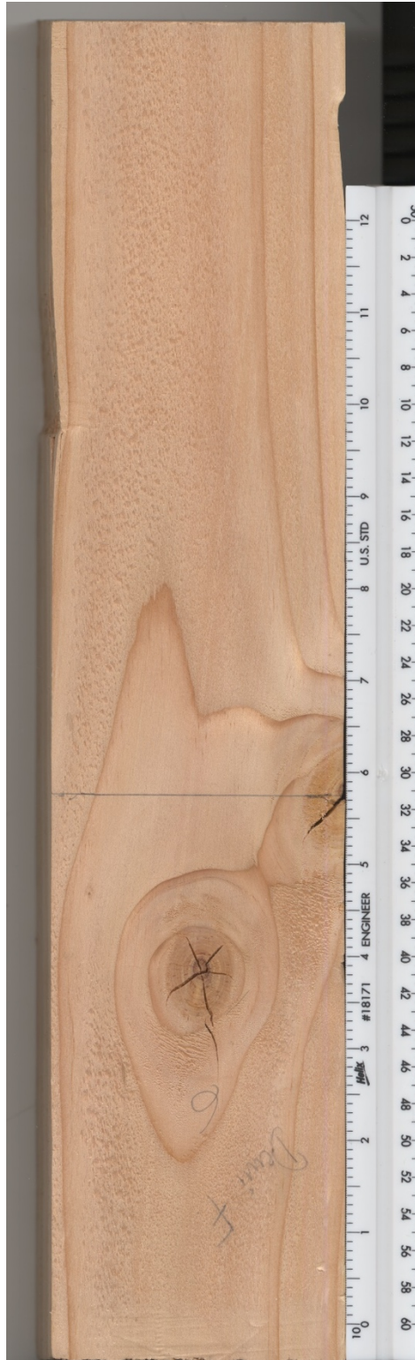
Figure 57. Specimen 3 of the Douglas fir Nuki joint of B_w = 1.5'' , scanned after rotational stiffness testing.
