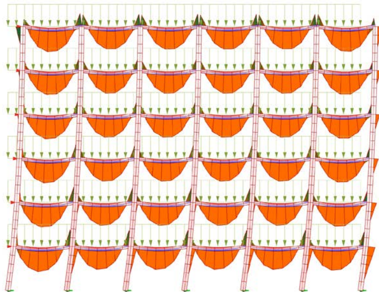
Figure 50. Preliminary assessment on the use of Nuki joints with rotational restraint for lateral systems, elevation view. 30 psf wind loads were applied as point loads assuming a 10 ft tributary width, as well as unfactored gravity loads outlined in Section 5.2. Timber columns measuring 20" x 20" were modeled.
