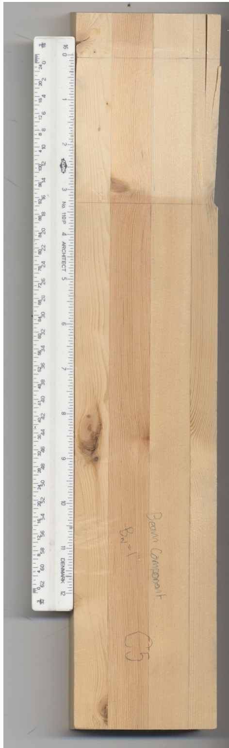
Figure 58. Specimen 5 of the glulam Nuki joint of B_w = 1'' , scanned after rotational stiffness testing.
