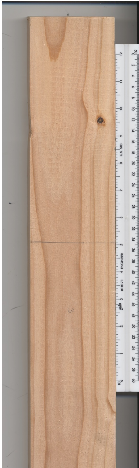
Figure 54. Specimen 3 of the Douglas fir Nuki joint of B_w = 1" , scanned after rotational stiffness testing.
