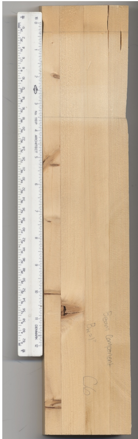
Figure 59. Specimen 6 of the glulam Nuki joint of B_w = 1" , scanned after rotational stiffness testing.
