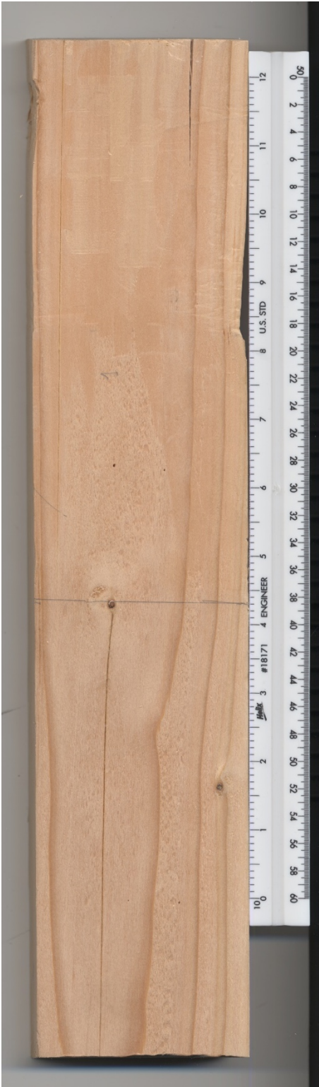
Figure 52. Specimen 1 of the Douglas fir Nuki joint of B_w = 1" , scanned after rotational stiffness testing.
