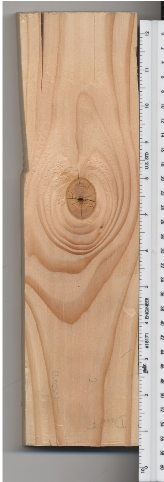
Figure 53. Specimen 2 of the Douglas fir Nuki joint of B_w = 1" , scanned after rotational stiffness testing.
