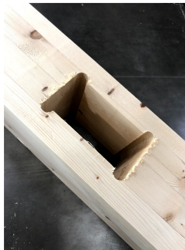
Figure 20. Mortise with rounded corners in the digitally fabricated prototypes.
