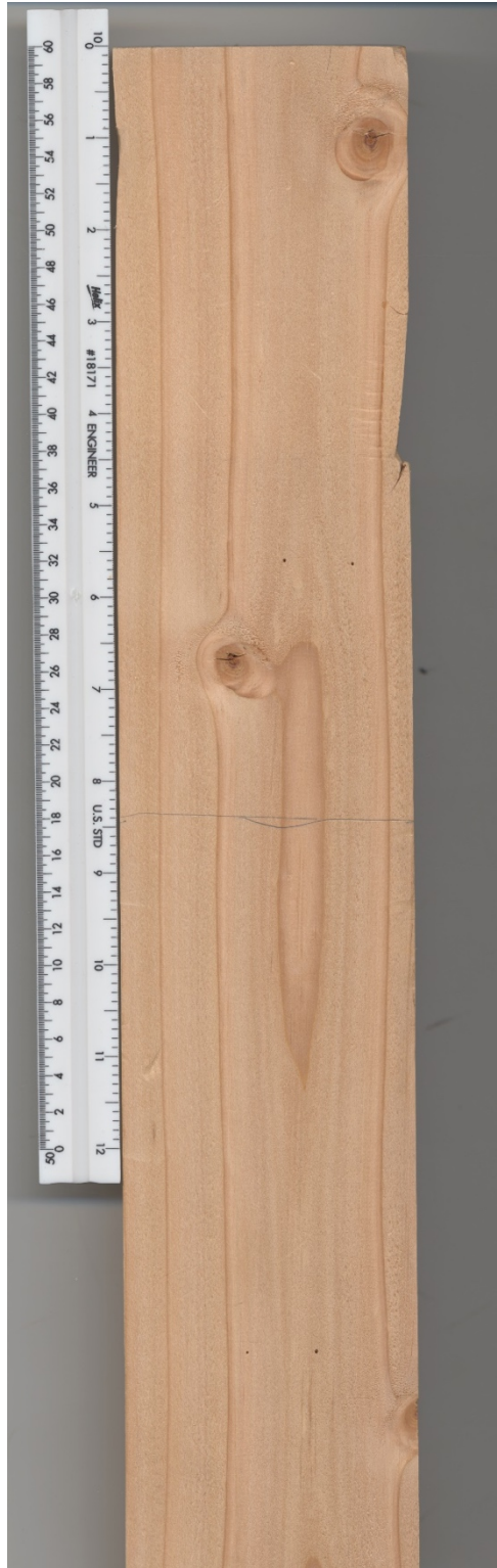
Figure 55. Specimen 1 of the Douglas fir Nuki joint of B_w = 1.5'' , scanned after rotational stiffness testing.
