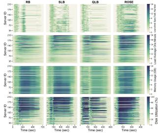
Fig. 14. Cluster resources utilization using oversubscription strategies. (Row#1: Launched speculative task number; Row#2: Load Average One Minute; Row#3: Memory usage; Row#4: Disk utilization;)
