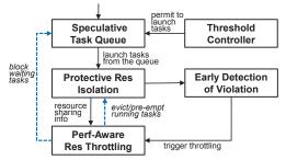
Fig. 9. Flowchart of resource throttling scheme
