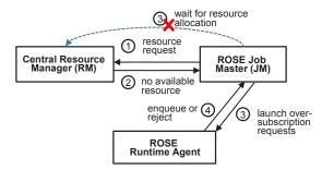
Fig. 4. Basic Idea of Speculative Oversubscription
