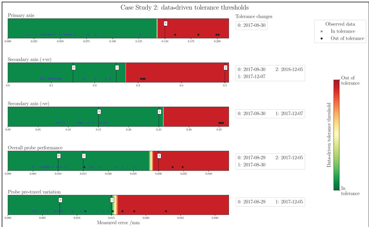
Figure 12. Case study 2: data-driven tolerance thresholds. From top to bottom: Primary-axis , Secondary-axis (+ve) , Secondary-axis (-ve) , Overall probe performance , and Probe pre-travel . Tolerance change occurrences in the data acquisition period are noted alongside each graphic.
