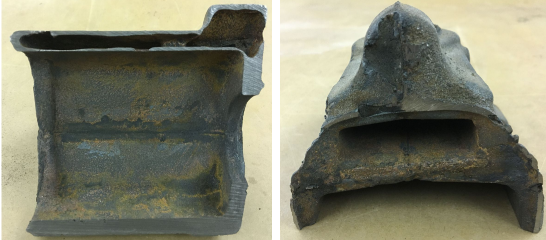
Figures 6-11 and 6-12: Two views of a manifold casting attempt, cut in half to show the void found within the thin wall; fabricated by Gordon Mosely P. Andrews, Spring 2016.
