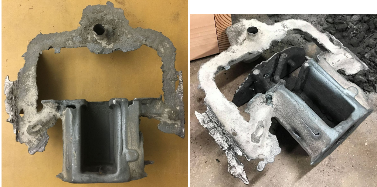
Figures 6-13 and 6-14: Left image showing manifold casting attempt, showing short shot; right image showing manifold casting attempt right after being broken out, showing the section of the core print that filled unintentionally; fabricated by Matt Quejada, Spring 2019.
