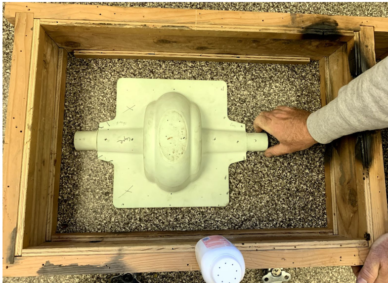
Figure 5-6: Placing the lower base pattern into the flask, making sure to leave room for the sprue. Talcum powder (baby powder) bottle shown sitting on the edge of the flask.
