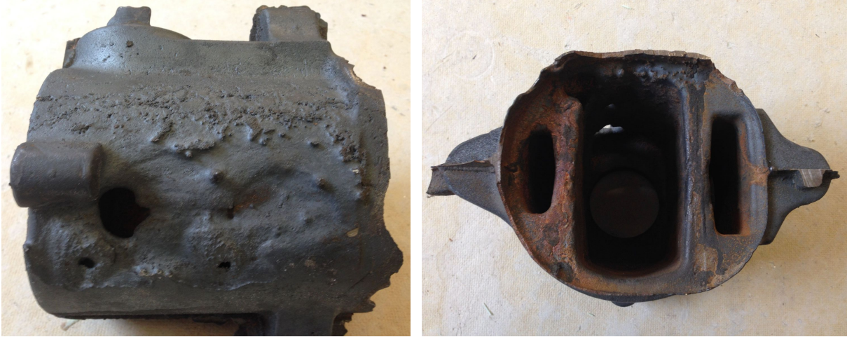
Figures 6-7 and 6-8: Two views of the first attempt to cast the manifold, showing the fill defect; fabricated by Gordon Mosely P. Andrews; Spring 2016.
