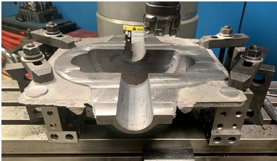
Figure 5-8: Lower base mounted to the bed of a 2-axis mill, supported and clamped on each corner by two 123 blocks; partially faced.
