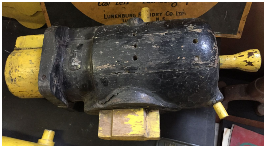
Figure 2-2: An example of a wood carved pattern, specifically the pattern for the Atlantic cylinder.
