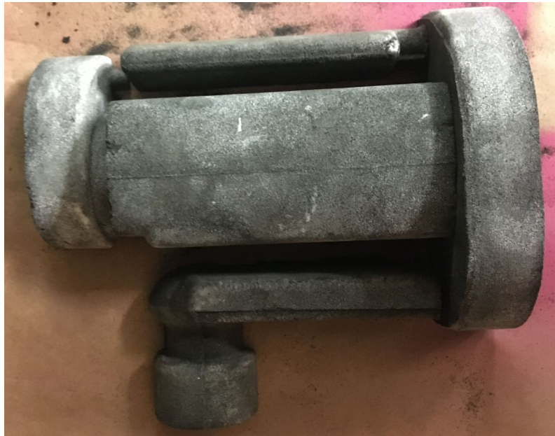
Figure 6-19: Half of the manifold core, created out of resin bonded sand using the redesigned core box.
