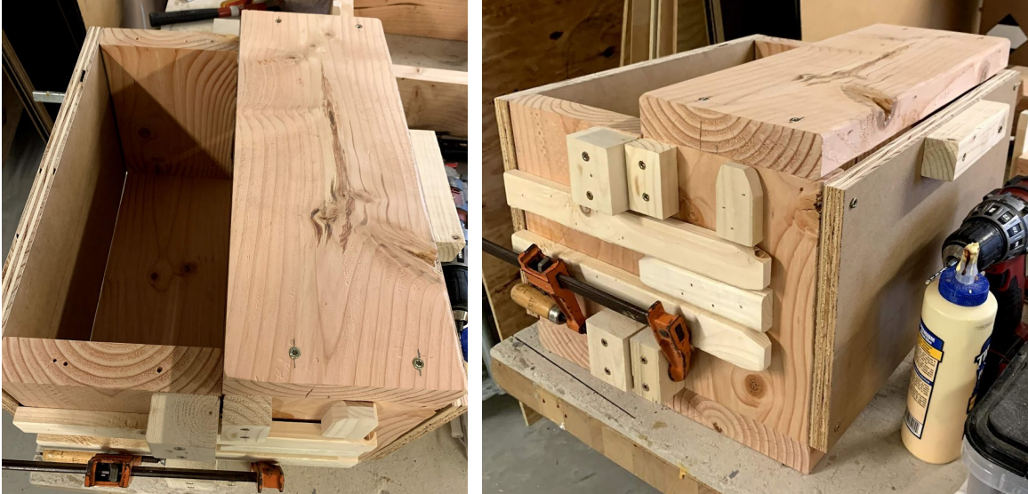
Figures 6-24 and 6-25: Left image showing a top view of the cope, with one of the top planks removed; right image showing the cope with one of the top planks removed, with a clear view of the interlocking and clamping mechanisms and the plywood side panel.
