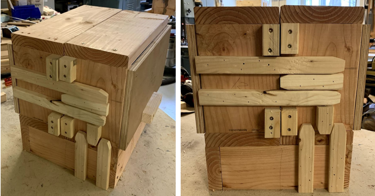
Figures 6-27 and 6-28: Two different views of the fully assembled three-part flask, showing the interlocking locating features, clamping surfaces, and the additional plywood panels.
