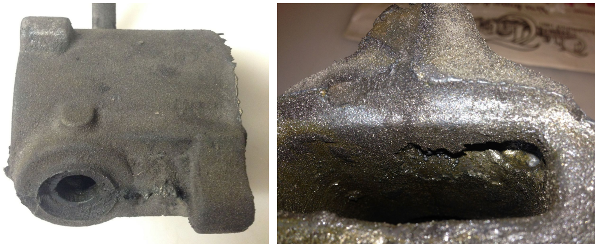
Figures 6-9 and 6-10: Left image showing the decreased flash on the second casting attempt; right image showing the internal cavity defects; fabricated by Gordon Mosely P. Andrews; Spring 2016.
