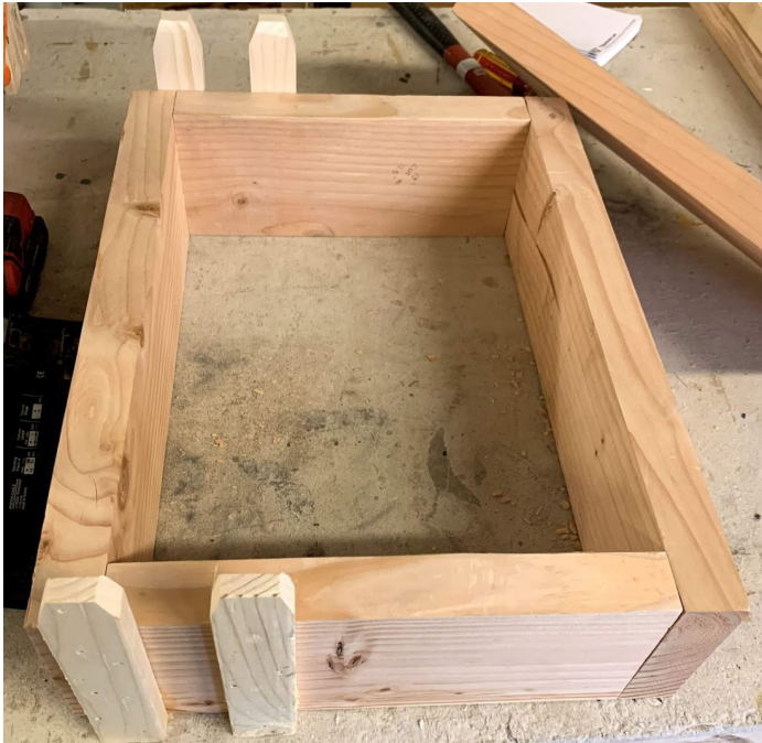
Figure 6-26: The drag component of the three-part flask.
