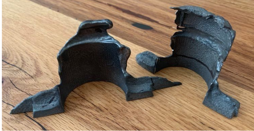
Figure 5-7: Core print flash removed from the casting; the more reflective areas being visible indicators of hardened sections due to rapid cooling during casting.
