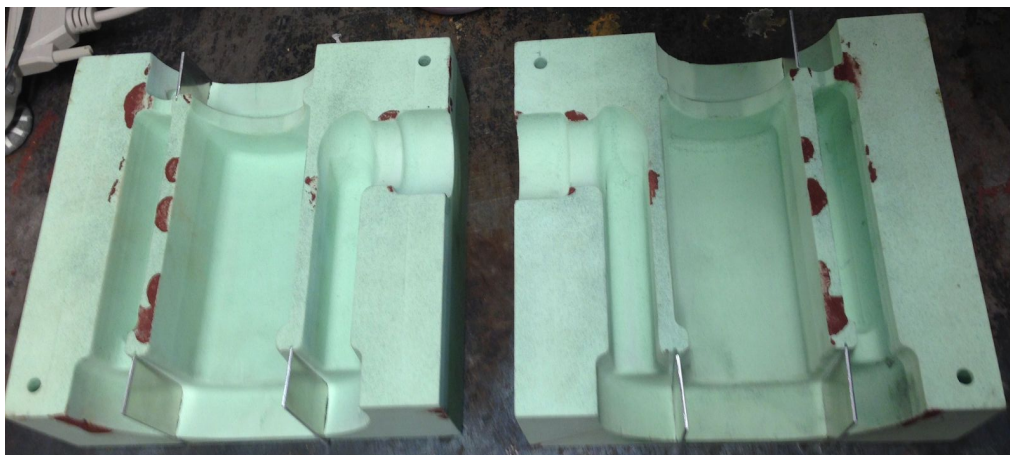
Figure 6-6: Modified manifold core box, adding metal shims to separate the different sections of the core; fabricated by Gordon Mosely P. Andrews; Spring 2016.
