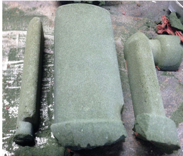
Figure 6-5: Broken core, created in one piece using the first iteration of the core box, but broken during removal, leaving rough interfaces between components.
