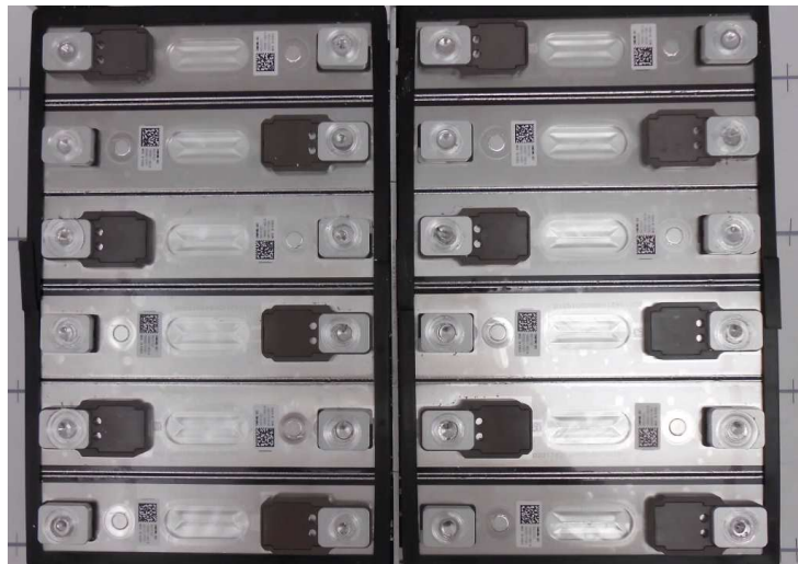
Figure 2-27: BMW i3 battery module [92]
