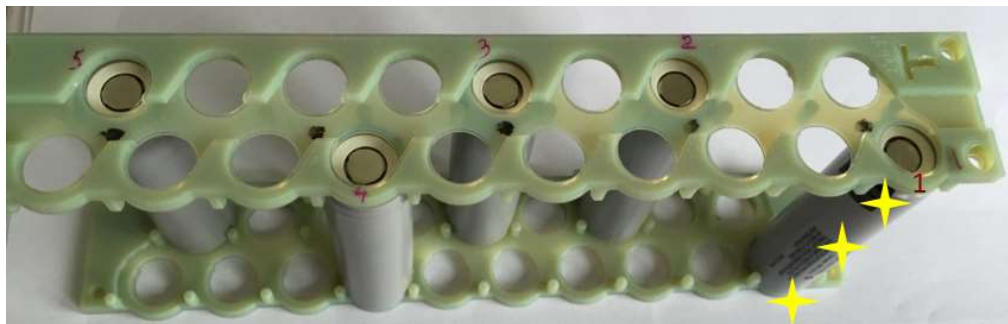
Figure 3-10: Temperature monitored cells within a 19 cell module
