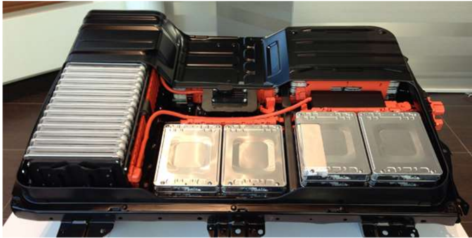
Figure 2-2: Nissan Leaf battery pack [58]
