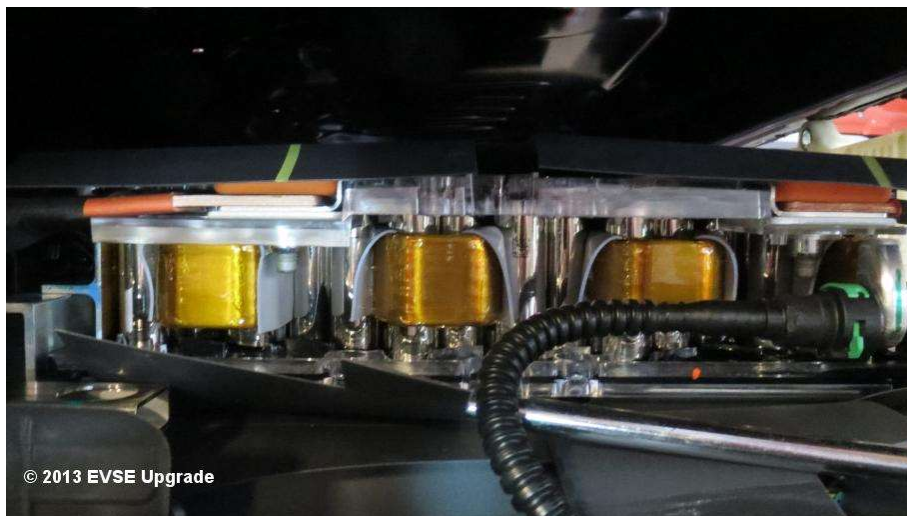
Figure 2-18: Tesla Model S cooling jacket [81]
