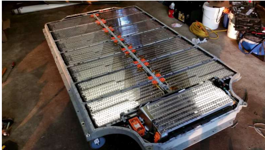
Figure 2-17: Tesla Model S battery pack arrangement [81]
