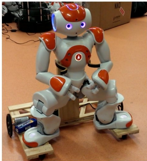
Figure 1: A Nao robot mounted on the robotic vehicle. The mounting bracket supports the weight of the torso while the foot-rests prevent the feet of the Nao from dragging on the floor while the Naos leg motors are disabled.
