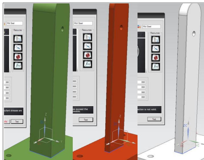
Figure 27 Bracket configurations; green for acceptable, red for wrong and white for unknown parameters
