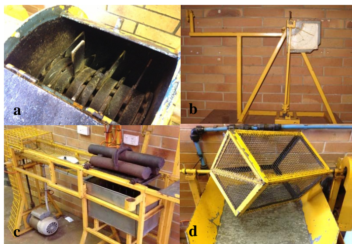
Fig. 3 —Equipment used to measure fibre quality components; a) hammer mill for cane preparation, b) impact resistance, c) shear strength and d) short fibre content.
