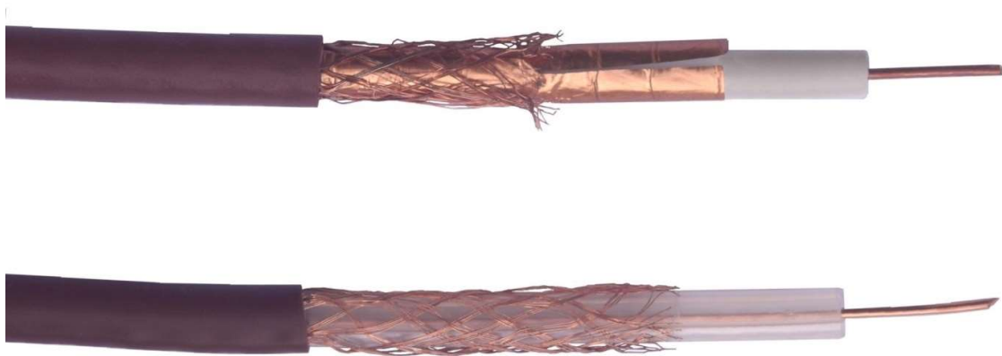
Figure 2 – Low-loss cables tested in this study: braid and foil (top), low coverage braid (bottom)
