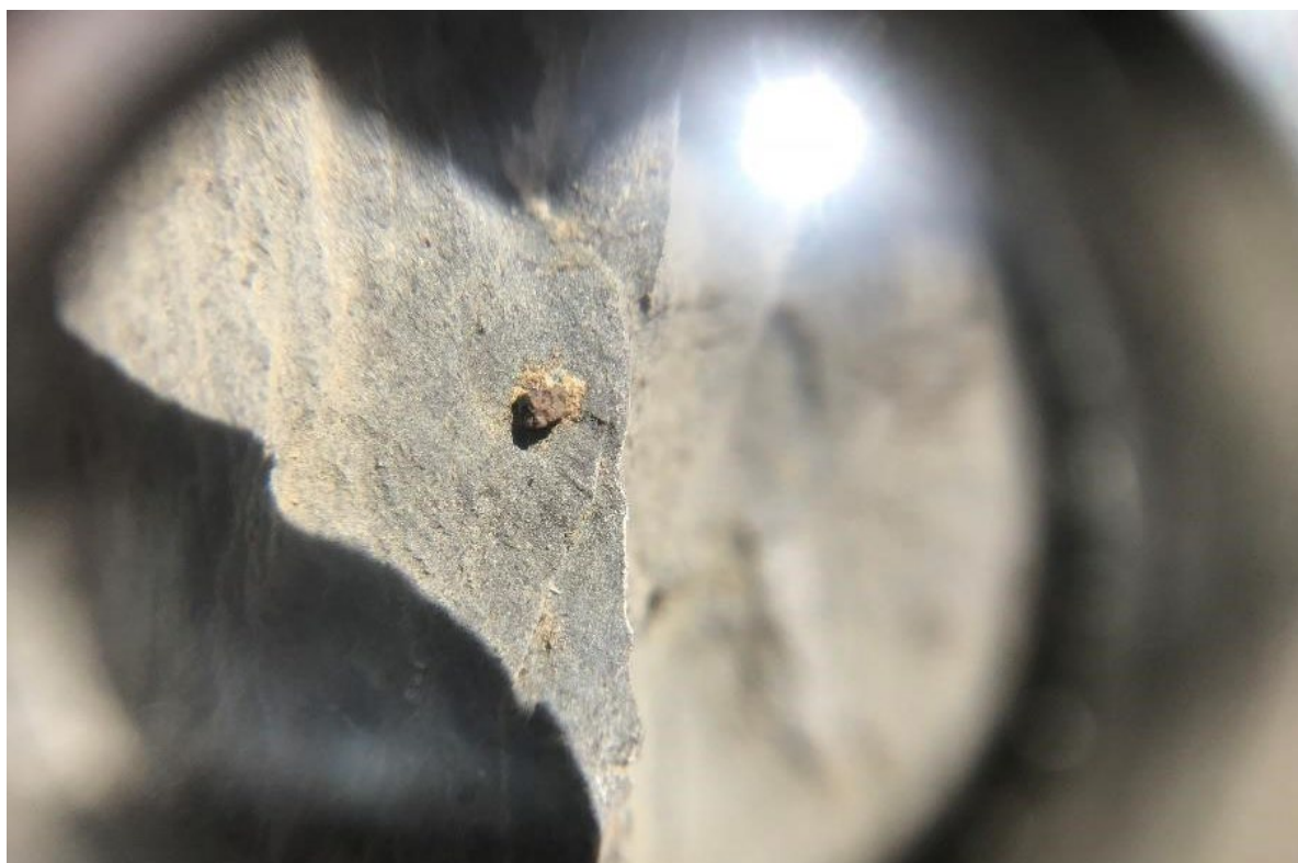
Figure 3.25 The High Pike Shelly Limestone Fmt. GR: 28154, 96905. Cuboidal grains with a metallic lustre can be observed coating the outside of the well weathered member.
