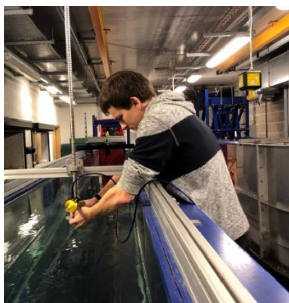
Figure 9: Changing the depth of the Valeport Impeller during the depth velocity calibration.
