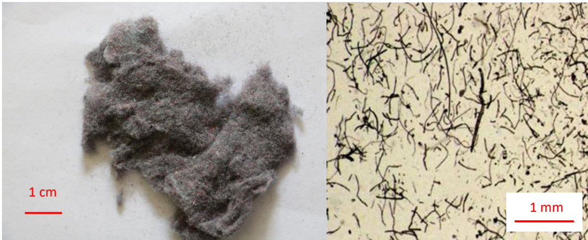
Figure 1: Illustration of a cutting of lint after manual removal of extraneous material and a microscopic image of resulting fibres.
