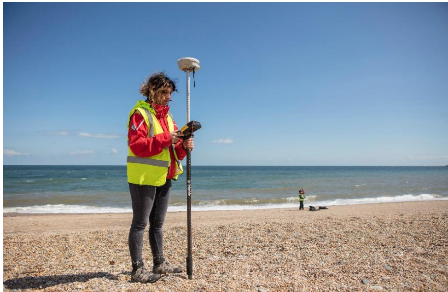
Figure 2.5. Surveyor with RTK-GPS survey pole conducting a 3D walking survey in Start Bay.
