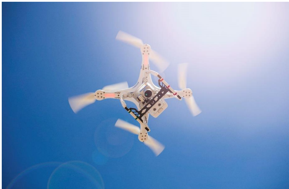
Figure 2.3. DJI Phantom Quad Copter, used throughout the study for sub-aerial surveys of Start Bay.
