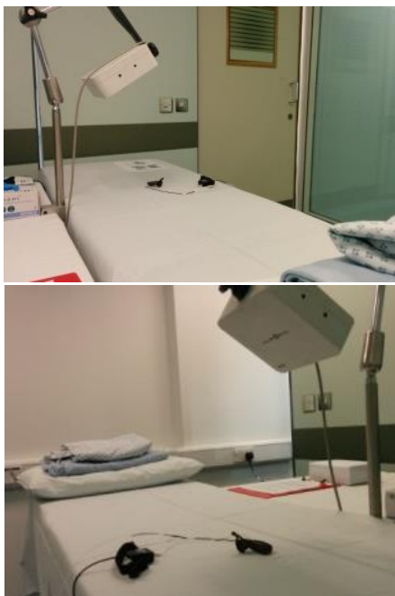
Fig. 1. Simulation environment for our experimental study. During each time slot, we recorded performance of a clinician doing two DREs on a RTA whilst wearing a position and a pressure sensor on the examining finger. The RTA wore a dressing gown and lay in left lateral position under the Aurora electromagnetic tracker.
