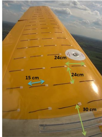
Figure 5: Wool tufts scheme on the upper surface of the wing.
