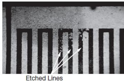
Fig 1-7 Microscope image of film resistor showing degradation of tracks [23].
