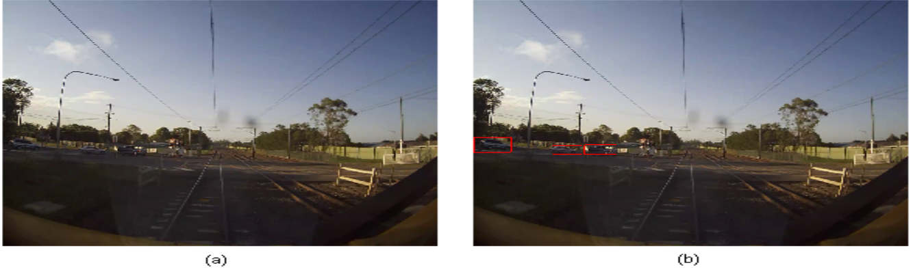
Fig. 8. Results of applying the vehicle detector algorithm to a cabin view at a railway level crossing. Subplot(a) shows a cabin view. Subplot(b) shows the position of the 3 cars that were detected by the vehicle detector.
