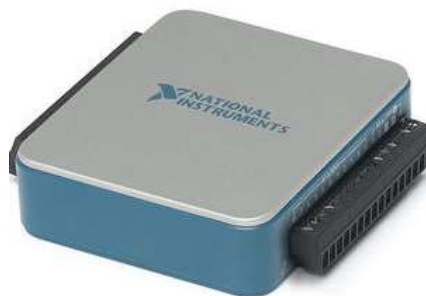
Fig. 4.16. A picture of a USB type data acquisition card (DAQ) card manufactured by National Instrument, which is used in our lab.
