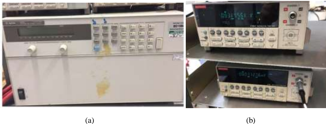
Fig. 5.3. (a) Power supply and (b) nanovolt meters for measuring the V - I curve of HTS coils.
