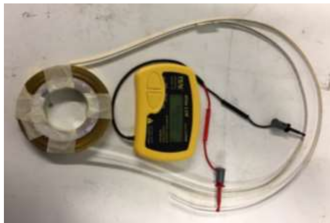
Fig. 5.5. Measurement of coil inductance ( L_{coil} ) of the INS REBCO coil via an inductance meter: “ atlas model LCR40 ” manufactured by PEAK electronic design ltd .
