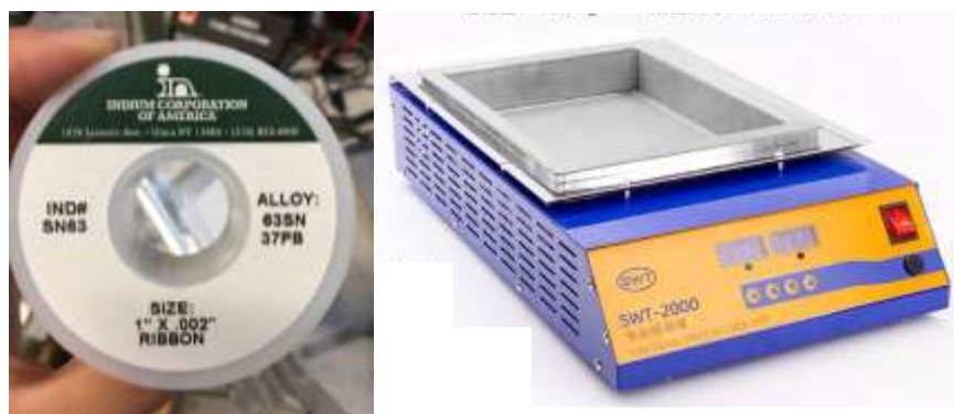
Fig. 5.8. Photos of the 6337 alloy (63% Sn (tin), 37% Pb (lead)) low temperature solder and solder pot for solder impregnation process.
