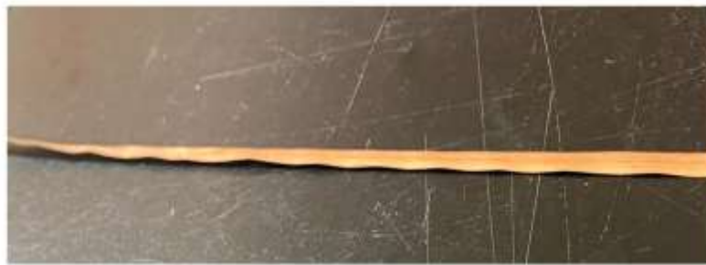
Fig. 2.19. The mechanical deformation at the edges of the REBCO conductors after test in a high field test coil for the 40 T superconducting magnet project at the National High Magnetic Field Laboratory (NHMFL), taken from [105].
