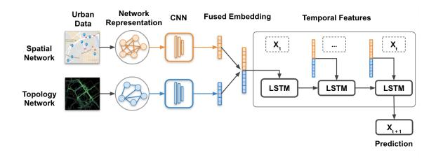
Fig. 5.3 An overview of the architecture to build spatial and topological representation of the venue graph which is then fed into a temporal model. Fed into the LSTM is the input and the previous hidden state.
