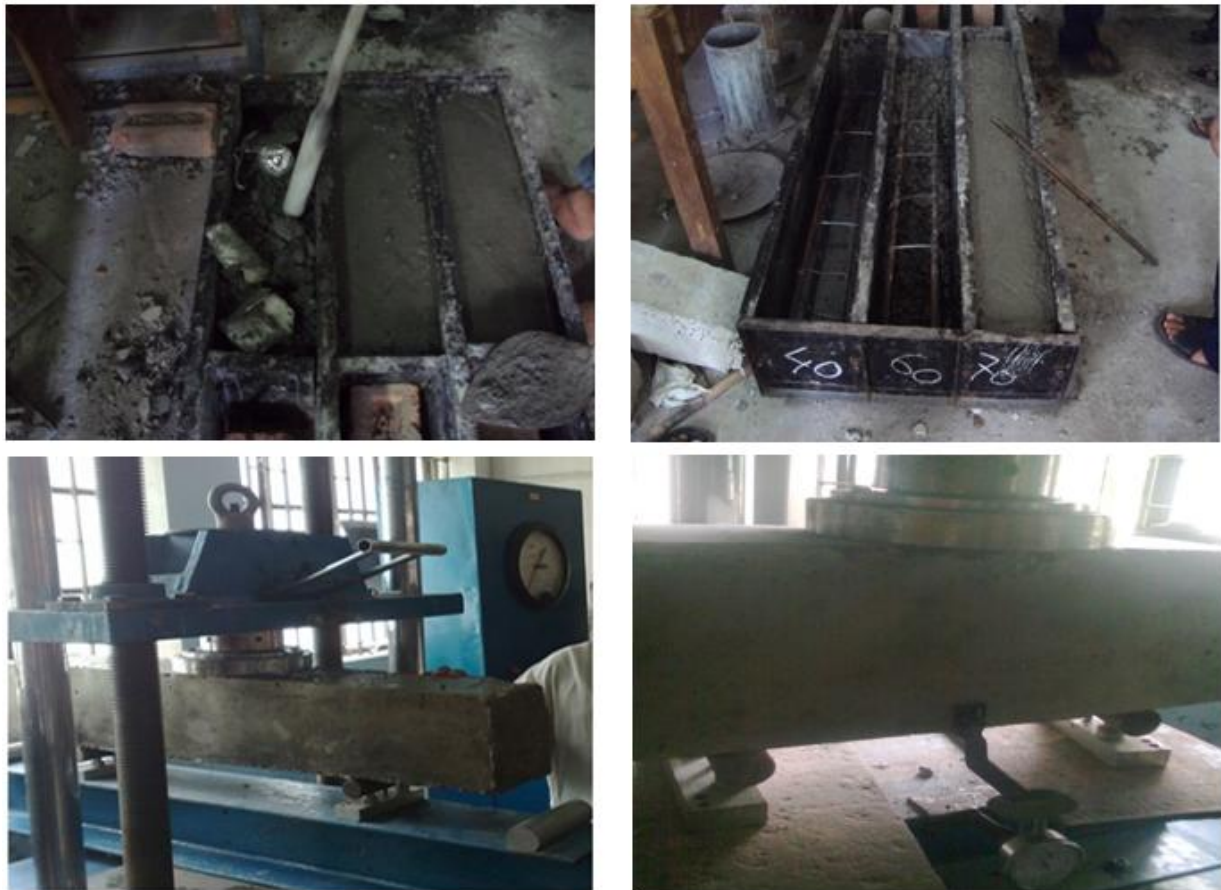
Figure 5: Short beam preparation and three-point bend test setup.
