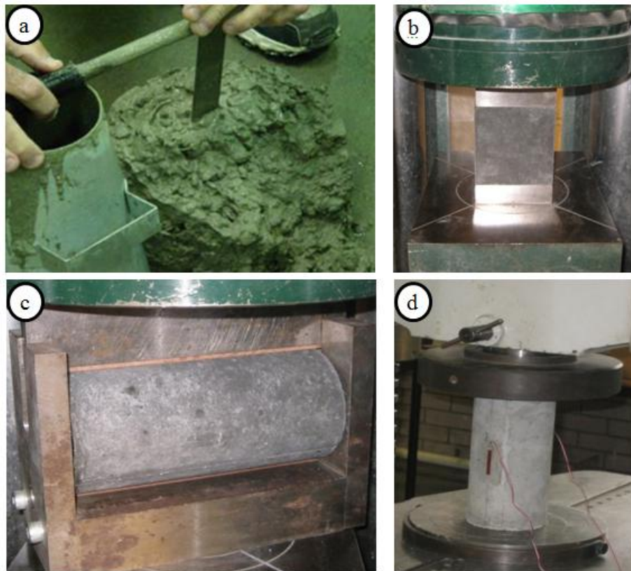
Figure 3: Typical a. Slump, b. compressive, c. tensile and d. modulus of elasticity test setup
