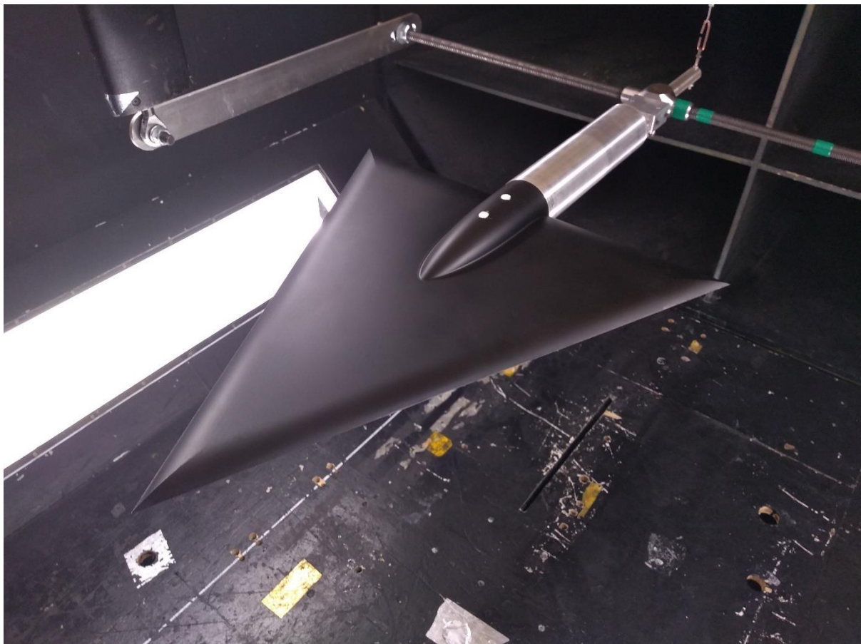
Figure 5.5 Looking down on the arrangement of the experimental rig in the wind tunnel at UWE Bristol showing the VFE-2 delta wing test model, and parts of the E-rig and strut support.
