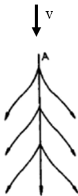
Figure 2.1 Pattern of attachment flows (Küchemann, 1978).
