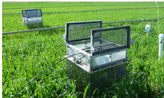
FIGURE 2 Automated chambers developed by Queensland University of Technology (Australia) in collaboration with Karlsruhe Institute of Technology (Germany). In this picture, standard 37.5-L chambers are atop 125-L extensions to accommodate wheat
