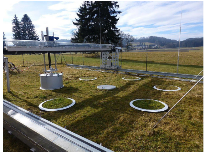
FIGURE 5 The Karlsruhe Institute of Technology Robotic greenhouse has chamber system for mounting on lysimeters at the DE-Fen site within the TERENO (TERrestrial ENvironmental Observatories) network
