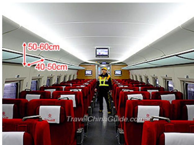
Fig. 12 Dimensions of hand luggage rack (TravelChinaGuide.com [31])
