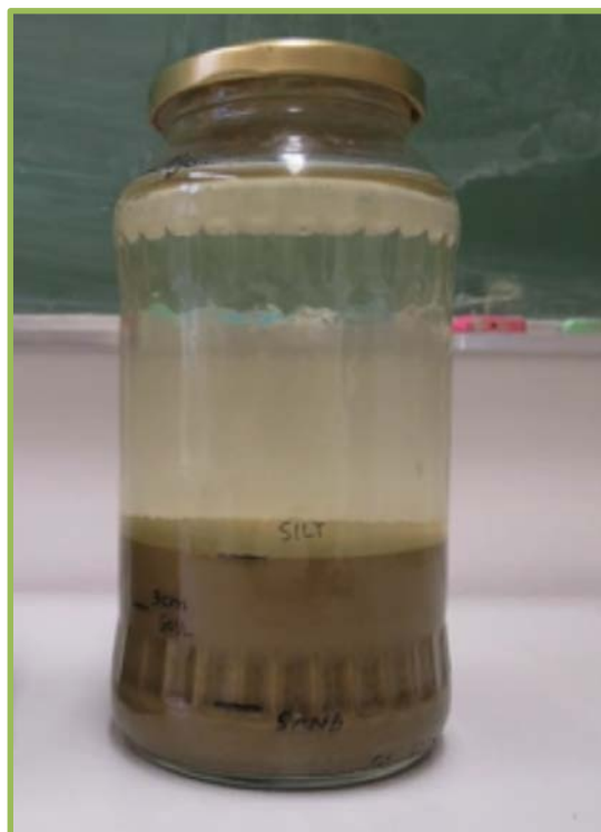
Figure 4.6 Sediment jar test showing settled layers (sand and silt are marked) and clear water
