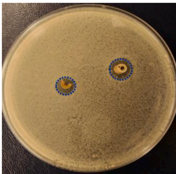
Fig. 3. Inhibition halo tests against S. aureus for PDA/CS/AgNPs-coated catheters after immersed into PBS solution for 30 days and then incubated in agar plate for 24 h.
