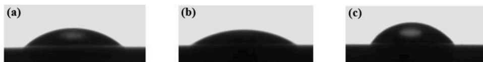
Fig. 6. Contact angle of a deionized water droplet on (a) uncoated Ti substrate, (b) PDA/CS-coated and (c) PDA/CS/AgNPs-coated Ti substrate.
