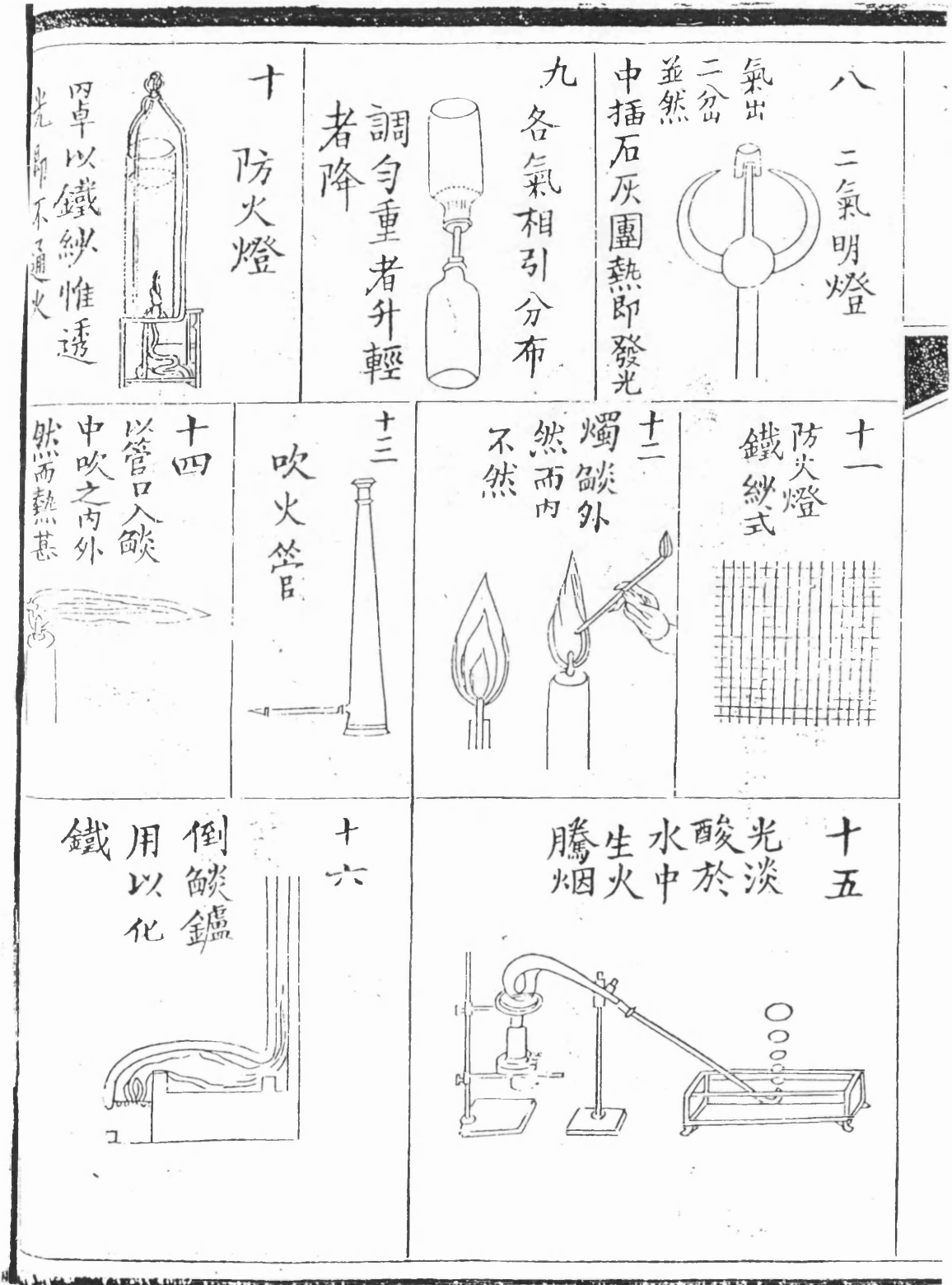
Figure 23. Illustrations of chemical equipment and processes from Gewu rumen . Top row, left to right: a safety lamp; diffusion of light and heavy gases; lime-light
