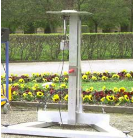
Fig 1. Measurement equipment (measuring lift, receiver's antenna)
