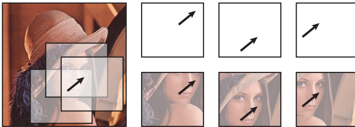
Fig. 1: The set of all translated windows exhibits stationarity since a single pair of pixels (indicated by the arrow) contributes to the statistics of all pairs with the same relative displacement. This results in a covariance matrix with Toeplitz structure, which Hariharan et al. [9] enforce to make estimation of the statistics of all windows feasible.
