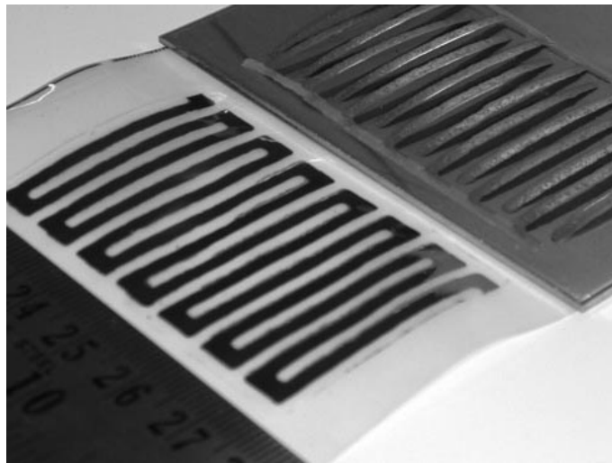
Fig. 2 Ni/Fe thermocluster structure and peeled PMMA masking ink
