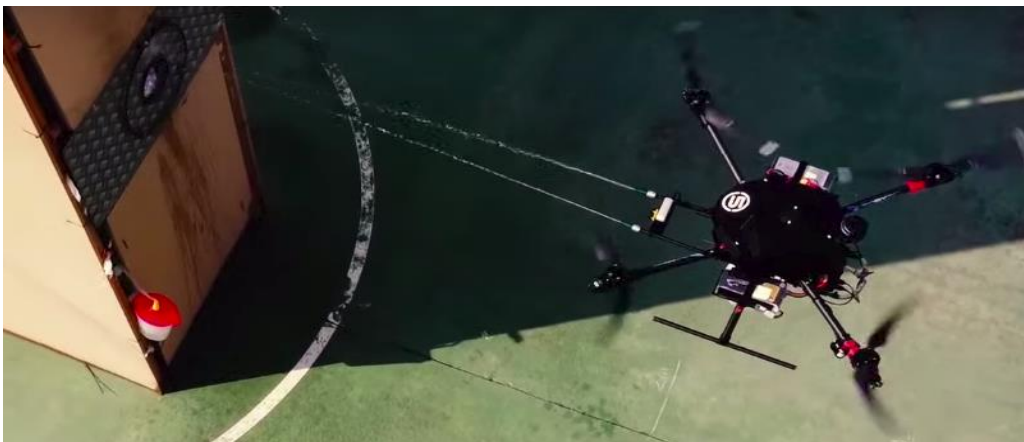
Figure 27: UAV Agent shooting water to the fire spot detected
