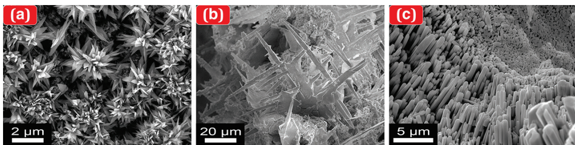
Figure 3.12 - Various nanostructures of metallic oxides produced by the SPSC method. (a) CuO nanoflowers ( UV_{24h} ). (b) CeO_2 dendrites ( Vis_{24h} , \lambda \approx 500 nm). (c) WO_3 nanorods ( UV_{48h} ).
