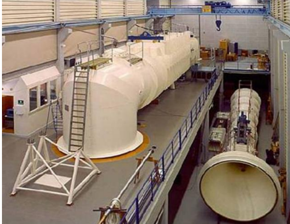
Figure 8 - The SSPA cavitation tunnel. Measurement section #1 to the right.
