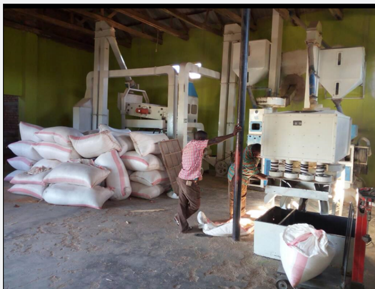
Figure 14. A small scale commercial milling line that accomplishes pre-cleaning of paddy, de-husking, polishing, and sifting to produce white rice separated into head rice, large broken rice, small broken rice, and fine broken rice in Igulusi, Mbarali district Tanzania. Photo credit: Christopher Mutungi/IITA.
