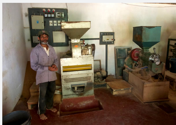
Figure 12. Two separate machines for two stage, two pass milling with rubber roller husker on the left and a steel polisher on the right. Photo credit: Retrieved from www.google.com .
