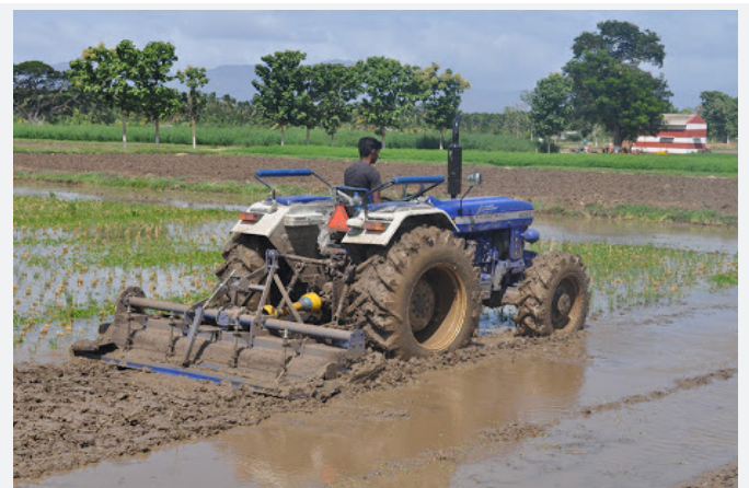
Picha Na.2.2. Kuvuruga udongo kwa kutumia trekta likikokota zana ya kuvuruga udongo. Picha imepatikana kutoka: website: https://www.quora.com/What-is-meant-by-puddling-in-agriculture .
