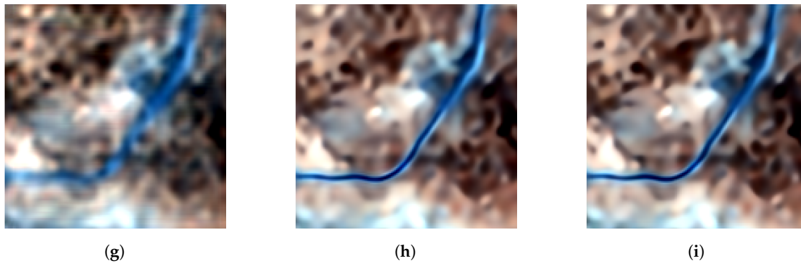
Figure 14. Results of a region of Teide 2017 from the W-S Set1. (a) HR, (b) LR with NN interpolation, (c) LR with bicubic interpolation, (d) SRCNN, (e) EDSR, (f) RCAN, (g) SRGAN with \alpha = 0 , (h) RS-ESRGAN ( \alpha = 0 ), (i) RS-ESRGAN ( \alpha = 0.1 ). Image size: 140 \times 140 pixels.
