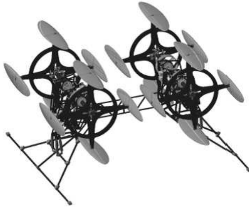
FIGURE 1.8: Designed cyclocopter with a total of 16 elliptic blades [32].
