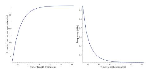
**Figure 3.4:** Maximum age of data and frequency of backup with change in timer length.  $\lambda = 0.07$ , slot length = 5 second,  $\alpha_i = \frac{i}{30}$ , and l = 20.
