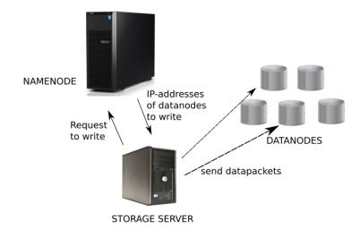
Figure 4.2: Data storage mechanism
