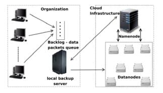
Figure 2.1: Components of the backup process
