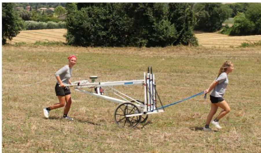
Figure 4. The magnetic gradiometry system LEA-MINI during the 2018 prospection at Monte Franco (Pollenza, Marche).
