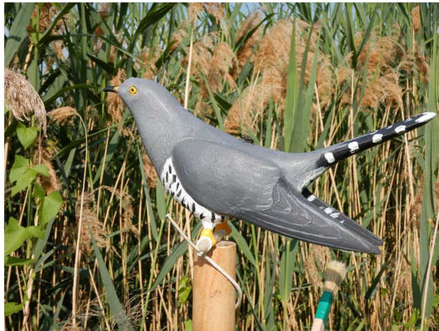
Figure 4. The 3D printed common cuckoo decoy used in our study. The decoy was painted with acrylic paint and mounted on a pole supplied with a noiseless electric motor to stimulate horizontal movement.
