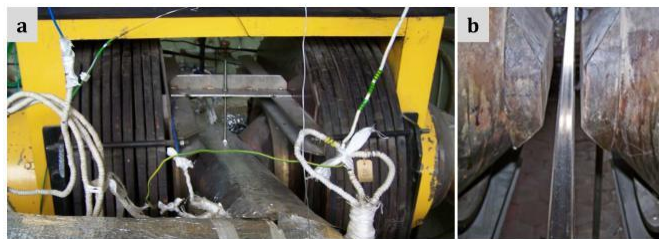
Fig. 12. (a) Experimental setup at the PbLi loop of IPUL. (b) Test channel installed between the magnet poles.
