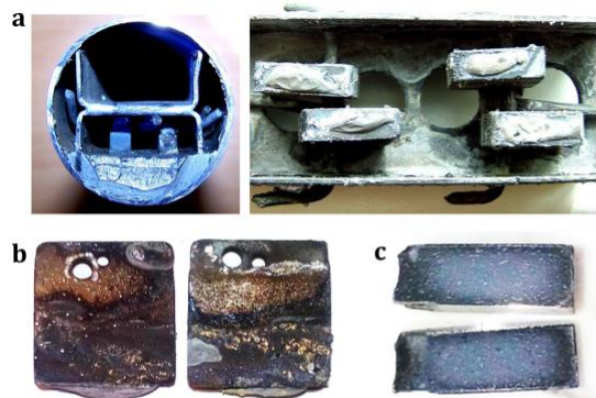
Fig. 10. Samples after the corrosion experiment under static PbLi. (a) In the experiment assembly. (b) Aspect of two samples, with PbLi adhered to the surface. (c) Cross sections of cut samples, where the inner porous SiC can be seen.
