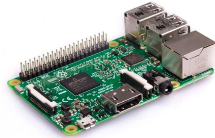
Figure 4-4: The outlook of raspberry pi 3B.[3]
