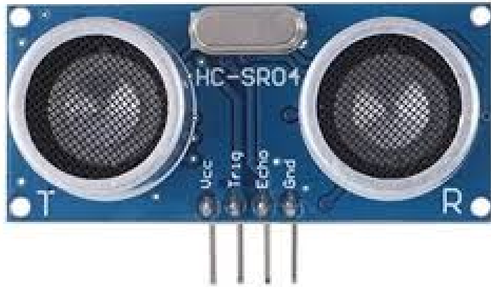
Figure 4-2: The main datasheet of HC-SR04 ultrasonic sensor.[1]
