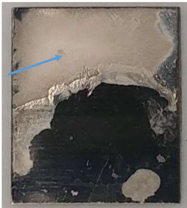
Figure 14. Pretreatment P. fluorescens biofilm on stainless steel substrate indicated by the blue arrow. Typically P. fluorescens film thickness is on the order of 2-15 \mu\text{m} . This image shows the biofilm after being dipped in DI water according to the experimental procedure outlined in Chapter 3.
