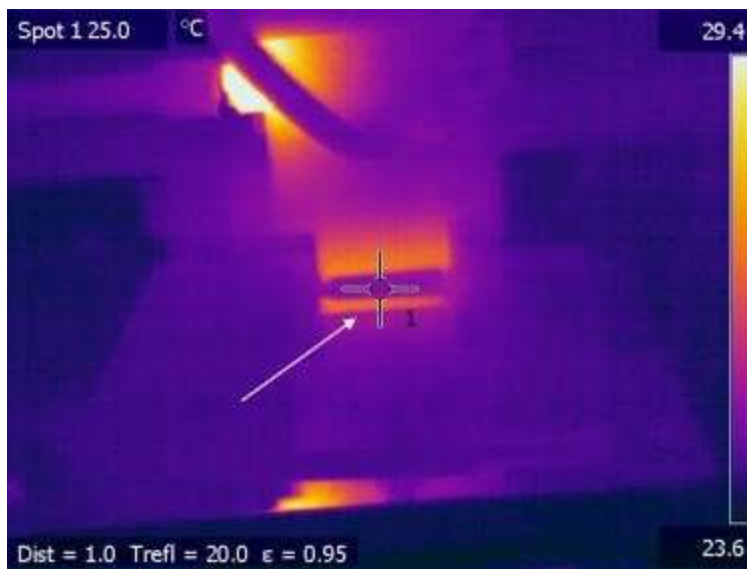
Figure 22. Thermogram of single linear discharge plasma device operating at 5 LPM Ar flow, 2 kV and 2.3 mA after five minutes of exposure. The gap between the electrodes is 1.2 mm and the device is 3 mm above the substrate. The temperature range shows the maximum and minimum temperature in the image to be 29.4°C and 23.6°C respectively. The steel heats only to 25°C which is far below the 35°C threshold.
