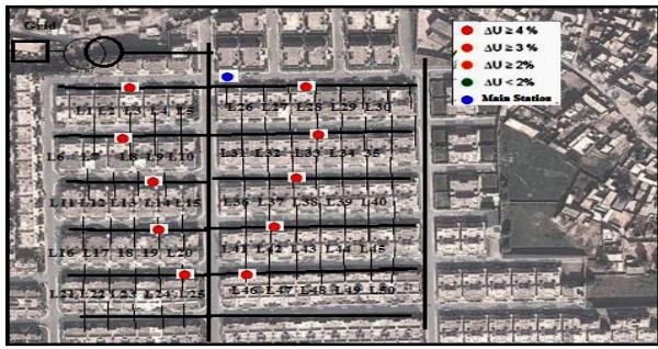
Figure 8: Selected 50 Houses load for Smart Grid
